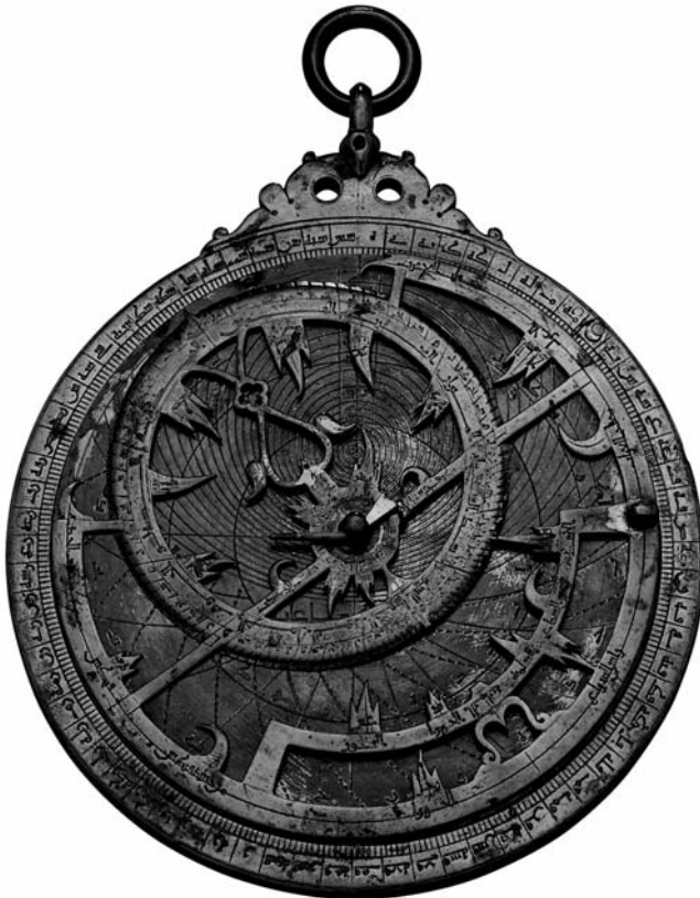
Figure 8.9. The front of a brass astrolabe made by Badr ibn ‘Abdallah ca. 1130 in Iran. 18.8 \times 13.4 cm. Note the rete star map and the tympan engraved with circles of altitude for the latitude of Persia. Courtesy of the Adler Planetarium & Astronomy Museum, Chicago, A-84. See also Color Section 3.
